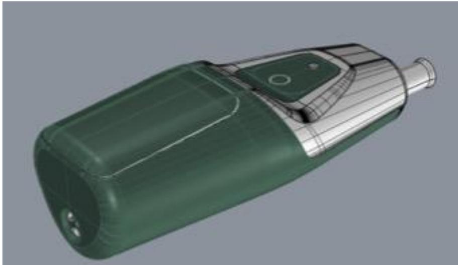
**Figure 1:** *The DSA COVID-19 Analyzer. The breath samples are given through a replaceable mouth piece (upper right hand corner), the outgoing air is filtered by a HEPA filter module (lower left hand corner). The device uses a local data network for communicating with the cloud applications.*
